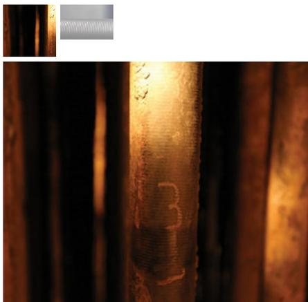
Pictured is a leading super heater tube from a test sample inspection. Boiler inspection was performed after approximately 14 months of operation. No shielding was installed on test samples. This image was taken after a water wash cleaning of the super heater tube.
